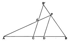
Draw any straight line through the point C, and take on it two points A', B', so that the ratio of CA': CB' is equal to the given cross ratio. Let the lines AA', BB' meet in P, and let PDbe drawn parallel to A'C meeting AB in D. Then D is a point such that the range  $\{AB, CD\}$  has the given cross ratio.
